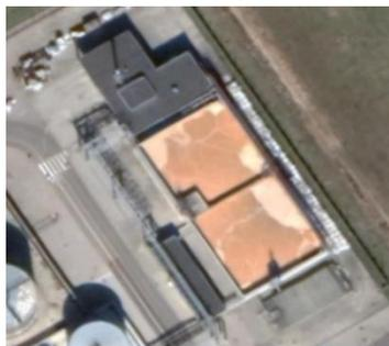
Fig. 6 Aerotanks – part of the biological cleaning equipment for wastewater
